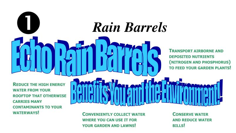
Throughout Arlington Echo we have Rain Barrels attached to the downspout of every building—adding up to 96 Barrels throughout campus. Rain Barrels gather the water that falls on the roofs and slows it down. The water from a 30 minute storm is released over 2 days.
